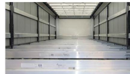
Beam spacing can be adjusted.
