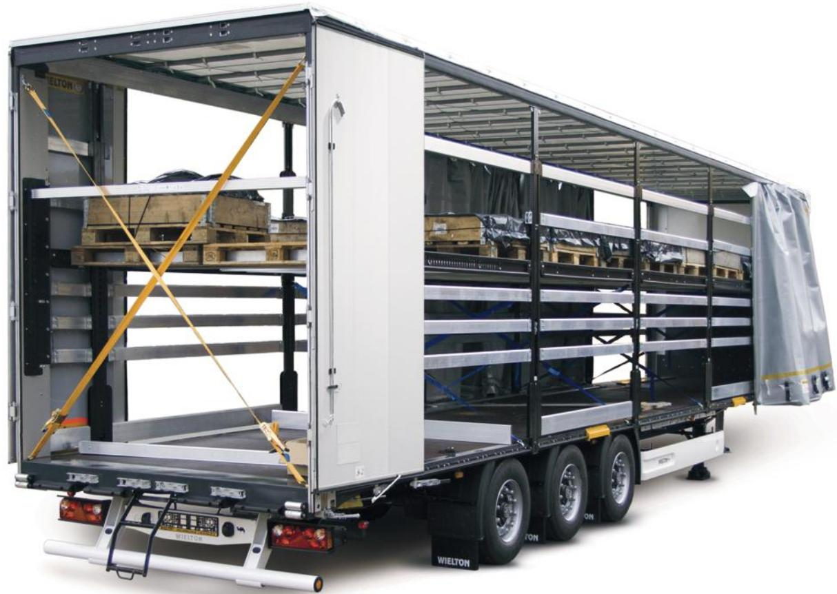
Arrangement of posts enabling easy loading.
