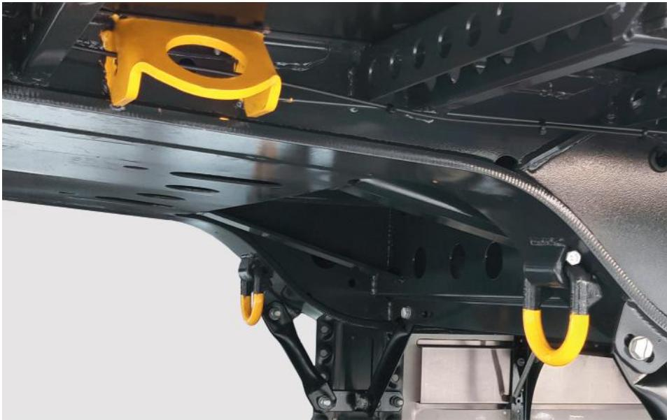
Floor mounting bracket (Coil Master).
