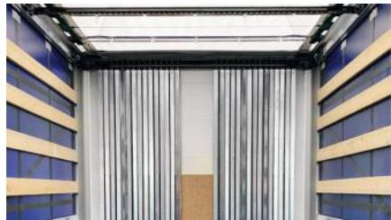
Vertical poles in unfolded position.
