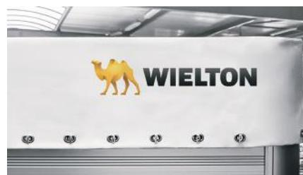
Improved tarpaulin construction and new, improved roof elements seal the cargo space, thus protecting the goods from moisture.
