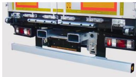
Pull-out support placed under the forklift.
