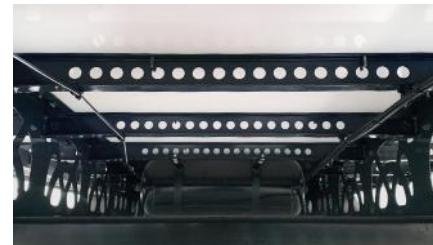
The reduction in overall weight of the new model has been achieved primarily through the use of alternative production materials such as high-strength S700 steel or the replacement of steel with aluminium in components such as air tanks, support legs, bumper, side buffers, etc.
