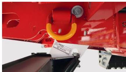
Marking of the places of securing the semi-trailer.
