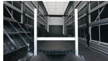
Frame adapted to transport of coils.
