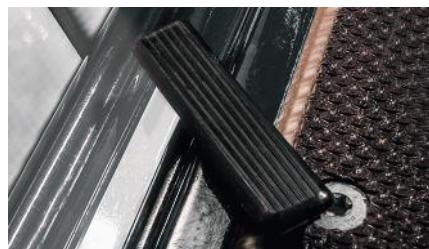
Smooth structure of the floor made of 30 mm board and additional plugs for holes on the frame in the place of cargo fixing.
